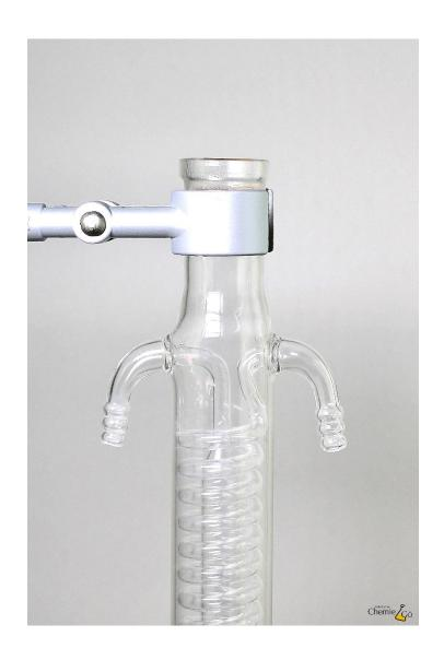
Reflux condenser are secured with a support clamp at the top ground-glass joint.
