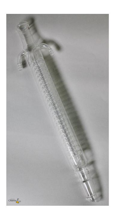
A coil condenser has a **cooling coil**.
