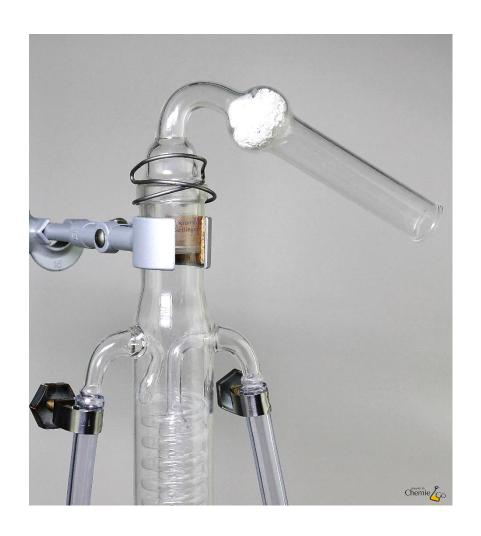
If the reaction mixture has to be protected from moisture, a filled drying tube is placed on the reflux condenser and secured with a clip. The cooling water is connected so that the entire cooling area is filled with water.
