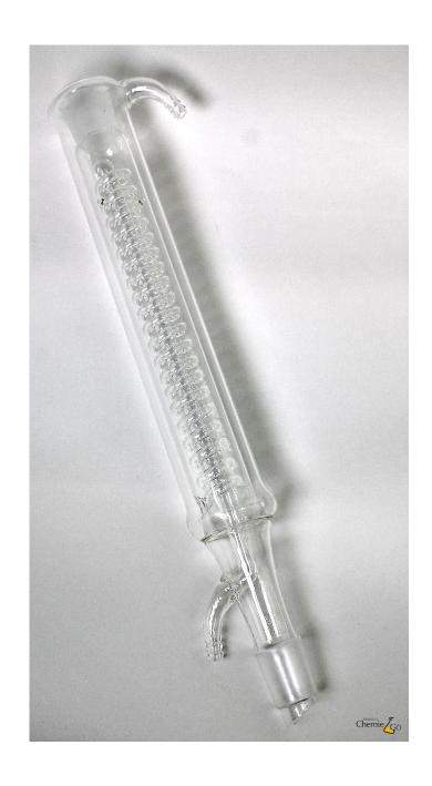
Jacketed coil condensers are used for special applications at very low boiling points.
